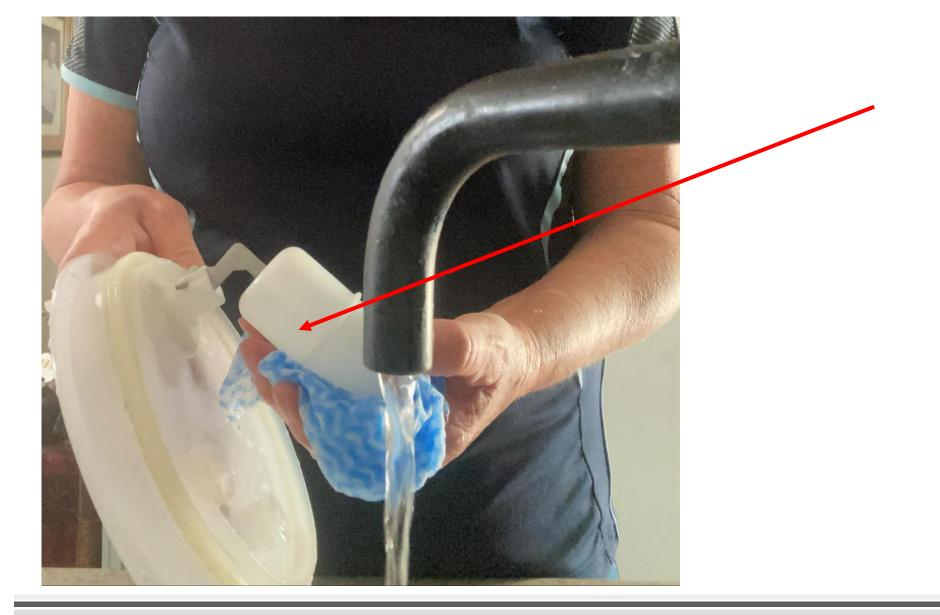
Clean plug and float by wiping it down with a clean chux, under some running water to remove any residue built up
