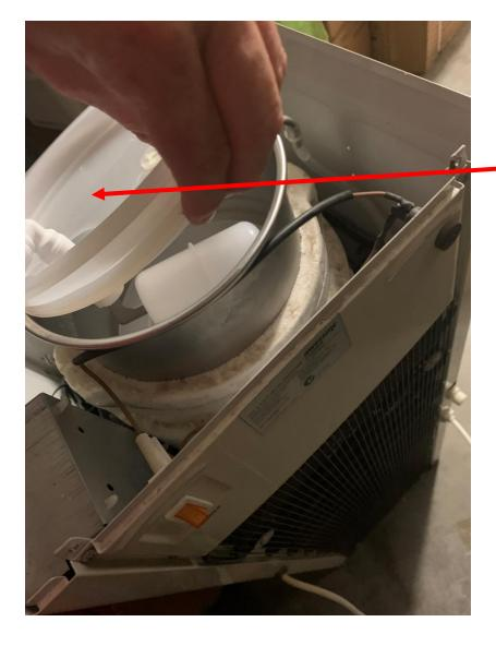
Remove the plug that sits in the tank by lifting it at one side, pulling upwards. Be careful as the edges of the tank is very sharp.
