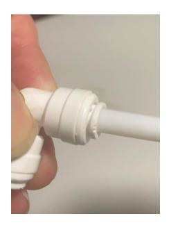
Push the pipe back as far as possible, and pull back on pipe to make sure it is locked in
