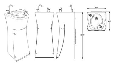
INLET: 860mm ABOVE BASE 100mm LEFT OF CENTRE LINE (from back) OUTLET: 860mm ABOVE BASE 30mm LEFT OF CENTRE LINE (from bac
